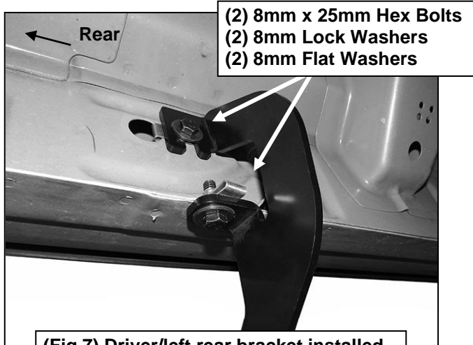
(Fig 7) Driver/left rear bracket installed
