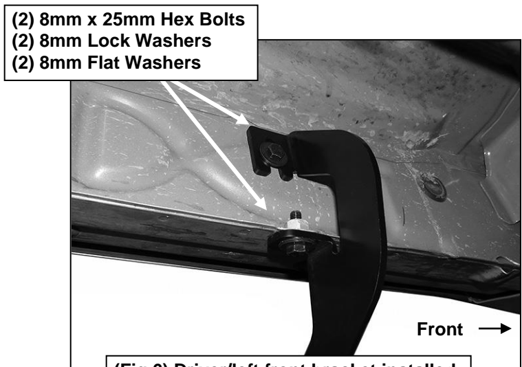
(Fig 6) Driver/left front bracket installed
