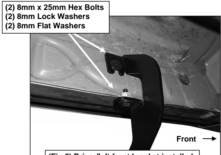
(Fig 6) Driver/left front bracket installed
