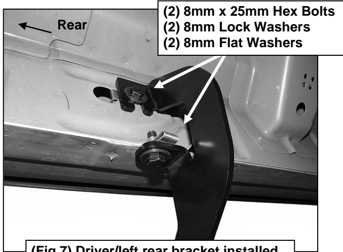
(Fig 7) Driver/left rear bracket installed
