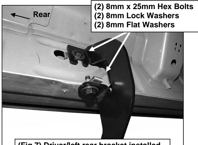
(Fig 7) Driver/left rear bracket installed
