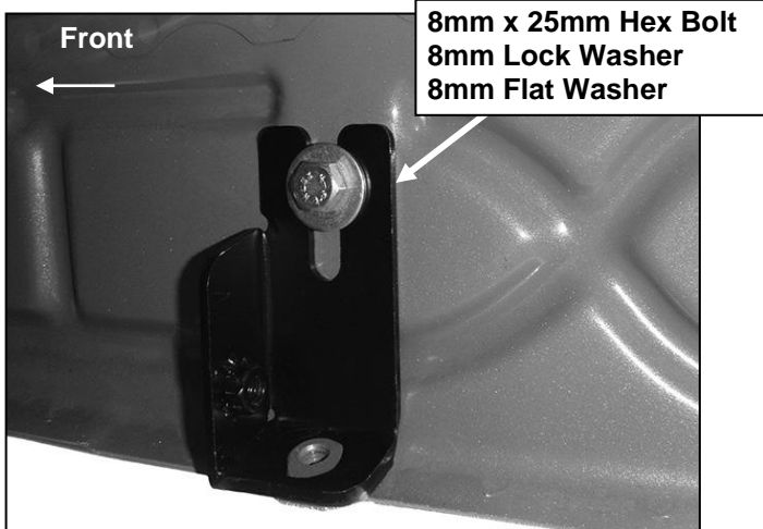
(Fig 11) Slide Upper Bracket over weld nut if equipped-also see Figure 2
