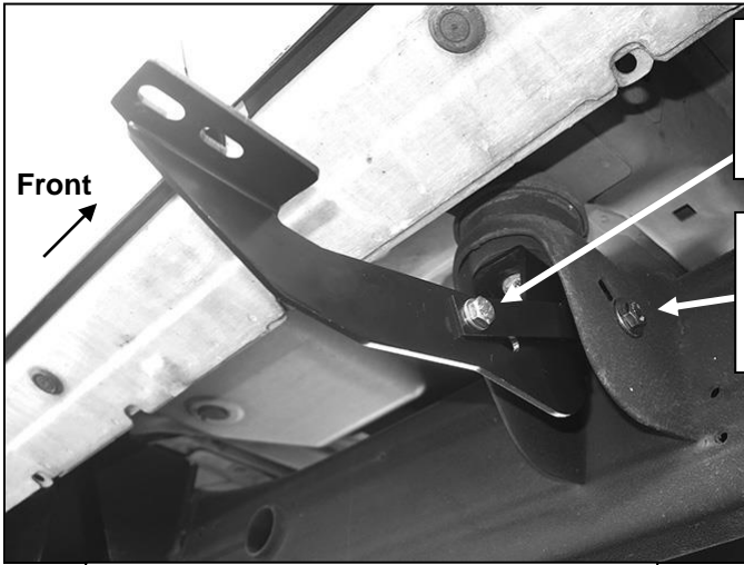
(Fig 10) Passenger side 25-3500 Model Center Support Bracket Installation
