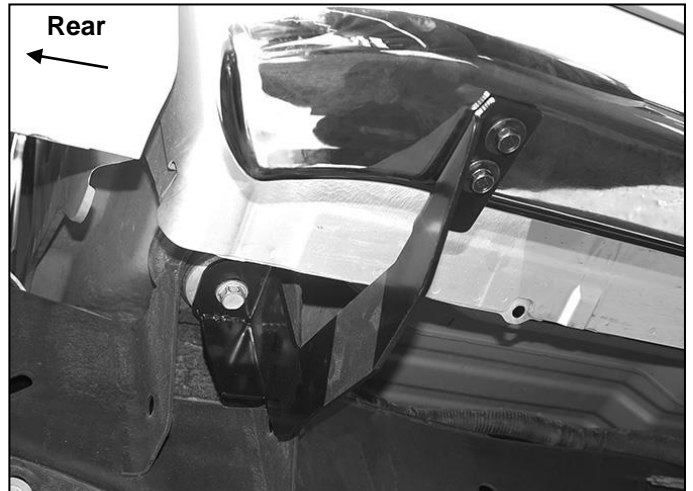
(Fig 11) Passenger side Rear Bracket Installation
