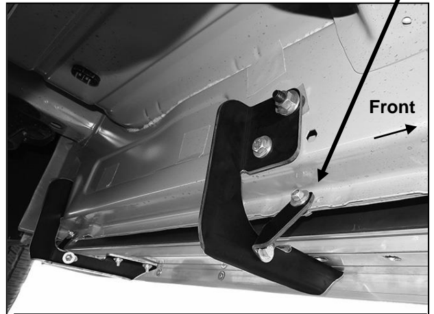
(Fig 14) Driver/left center and rear installation
