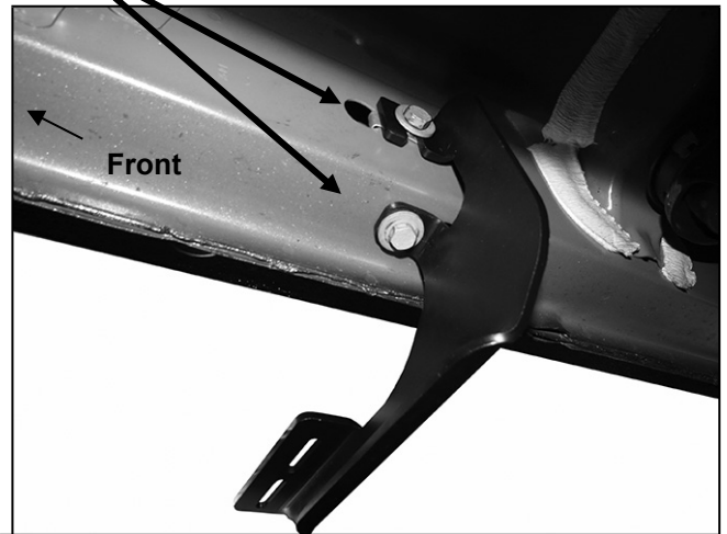
(Fig 4) Passenger side center Bracket installation
