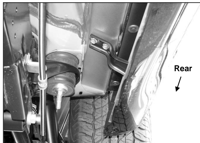
(Fig 3) Driver/Left Rear Mounting Location Pictured
