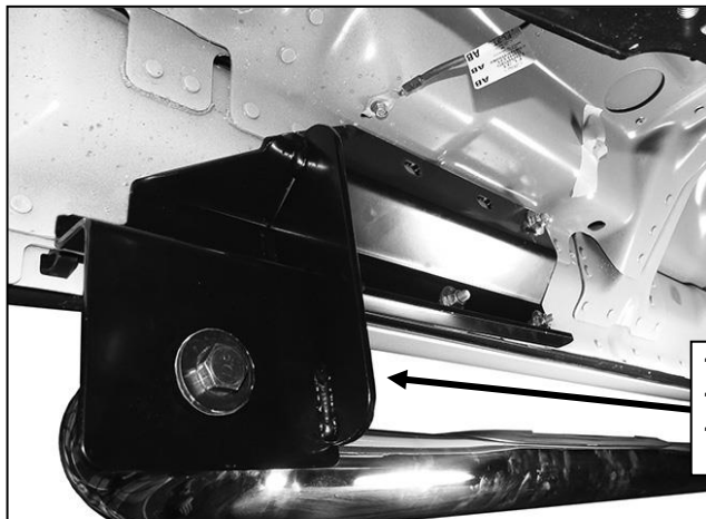
(Fig 5) Passenger side front Bracket installation
