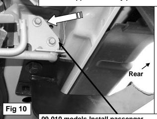
09-010 models-Install passenger side rear Mounting Bracket between exhaust support and body panel.
