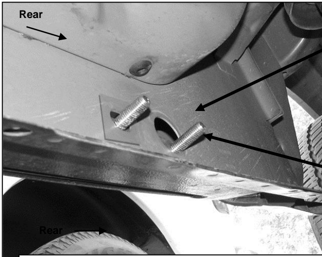
(Fig 4A) Passenger side rear mounting location pictured. Shown with Plastic Retainer in place
