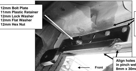
(Fig 3) Super Cab and Super Crew Cab passenger side Front Mounting Bracket pictured
