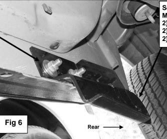
Secure the Sidebar to the Mounting Brackets with: 2) 1/2" x 2" Hex Bolts
