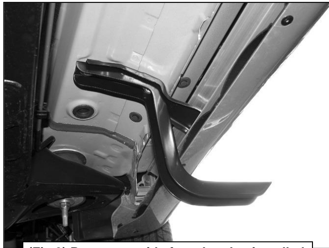
(Fig 3) Passenger side front bracket installed
