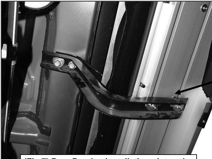
(Fig 7) Rear Bracket installation pictured
