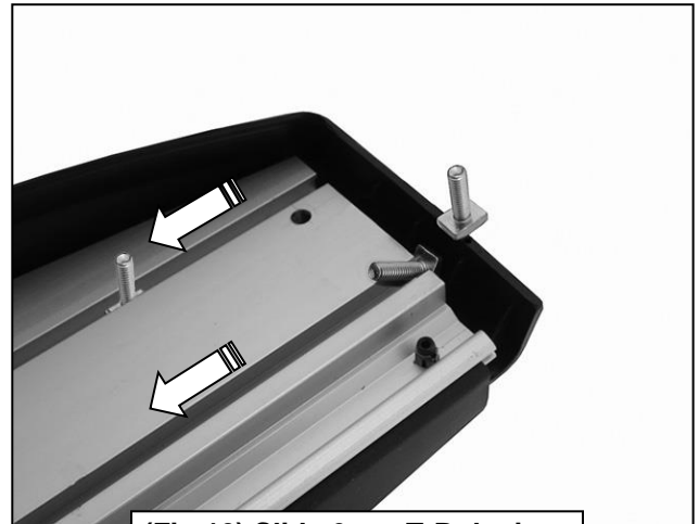
(Fig 10) Slide 6mm T-Bolts into slots at end of Running Board
