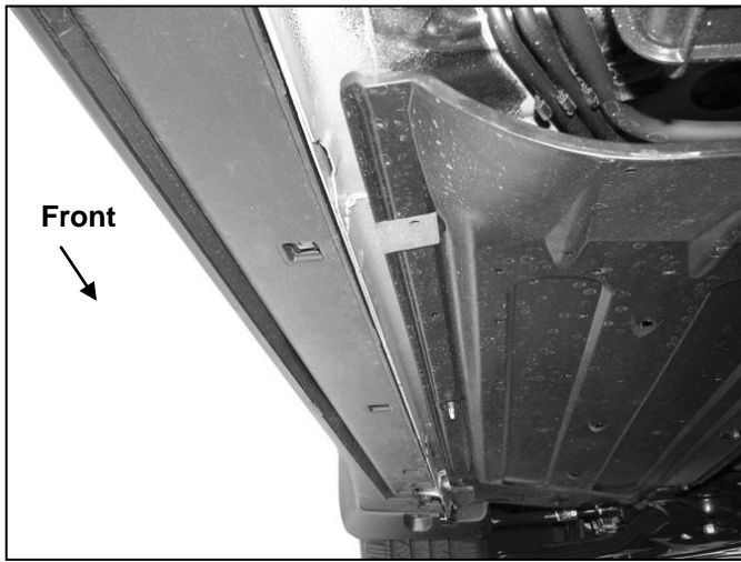
(Fig 8) Cut only enough to clear the Bracket. Reinstall the plastic cover
