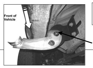
10mm x 30mm Hex Bolts 10mm Lock Washers 10mm Flat Washers Or Factory Bolts
