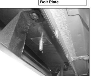
(Fig 3) Thread Plastic Retainer onto Bolt Plate
