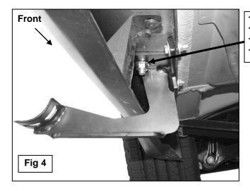
12mm Bolt Plate 12mm Plastic Retainer 12mm Flat Washer 12mm Flange Nut
