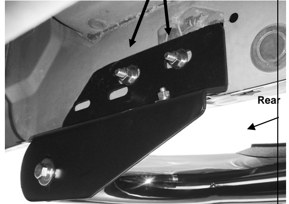
(Fig 4) Rear Mounting Bracket installation (except driver side Mounting Bracket on 97-98 3-door models)
