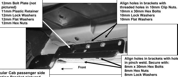
(Fig 3) Regular Cab passenger side **Front Mounting Bracket pictured**
