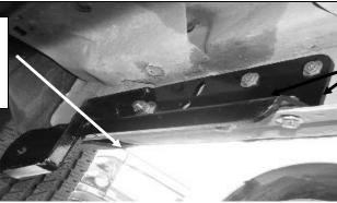
Align holes in brackets with threaded holes in 10mm Clip Nuts. 10mm x 30mm Hex Bolts 10mm Lock Washers 10mm Flat Washers
