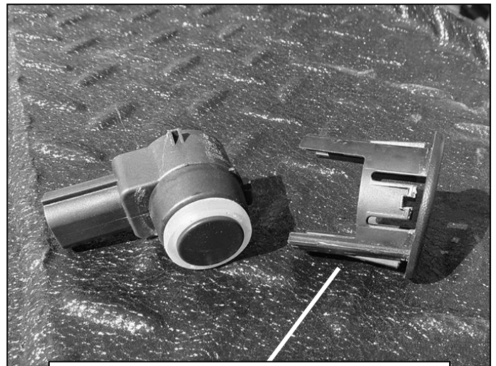
(Fig 2) Remove the mounting sleeve (right) from each sensor location in bumper
