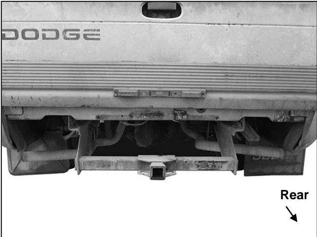
(Fig 3) Remove bumper and housing around license plate
