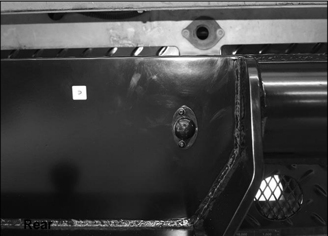
(Fig 5) Attach factory license plate lights to Bumper. Insert (2) Plastic Plugs for license plate
