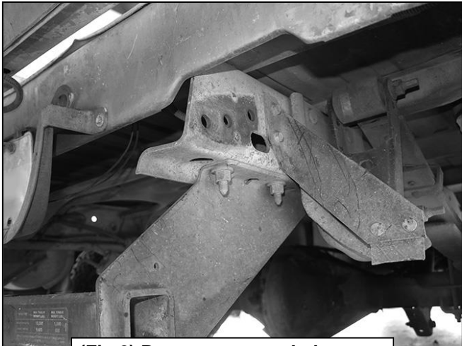
(Fig 2) Bumper removed, do not remove receiver hitch if equipped
