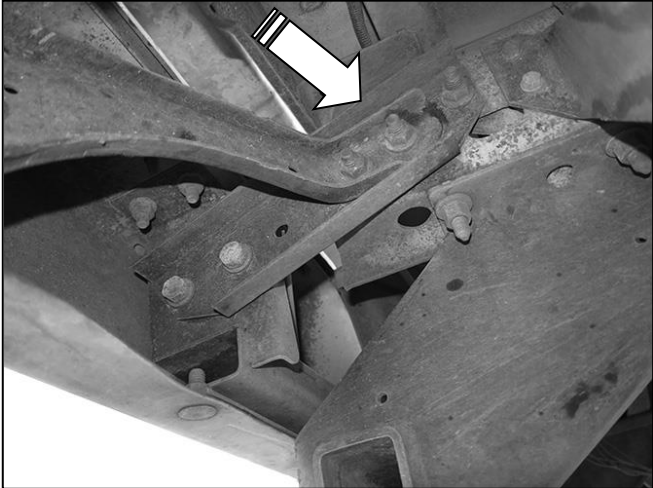
(Fig 1) Remove (3) hex bolts (arrow) from each side (passenger/right side pictured)
