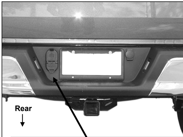
(Fig 1) Unplug and remove 7-wire trailer plug
