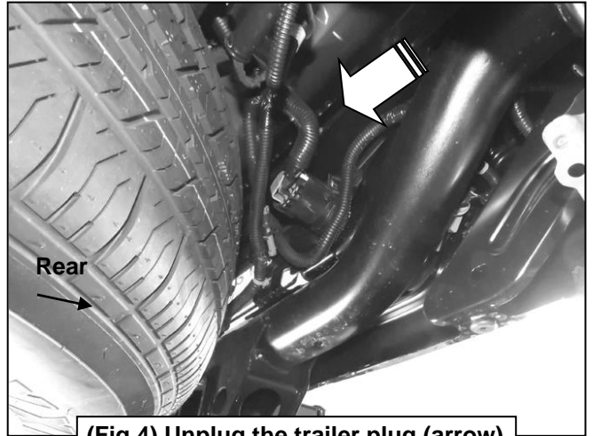
(Fig 4) Unplug the trailer plug (arrow)
