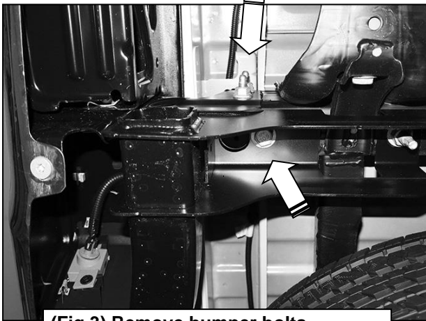
(Fig 3) Remove bumper bolts attaching brackets to frame (arrows)
