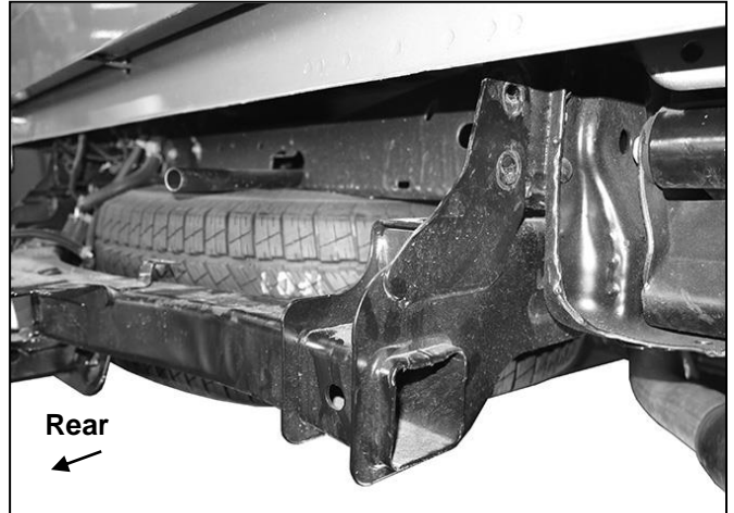
(Fig 4) End of frame once factory bumper is removed
