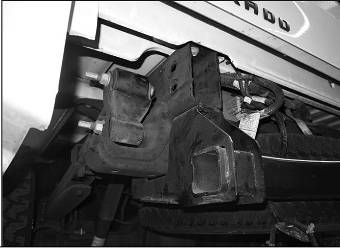
(Fig 3) End of frame once factory bumper is removed
