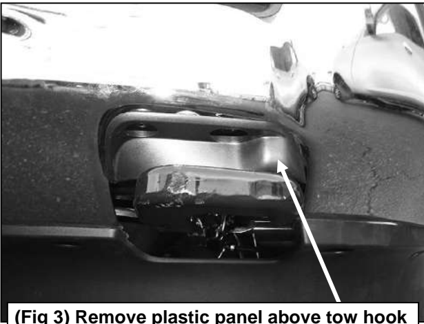
(Fig 3) Remove plastic panel above tow hook
