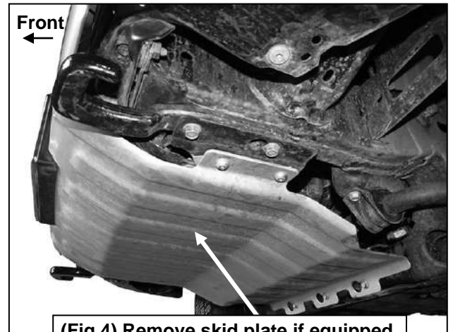
(Fig 4) Remove skid plate if equipped
