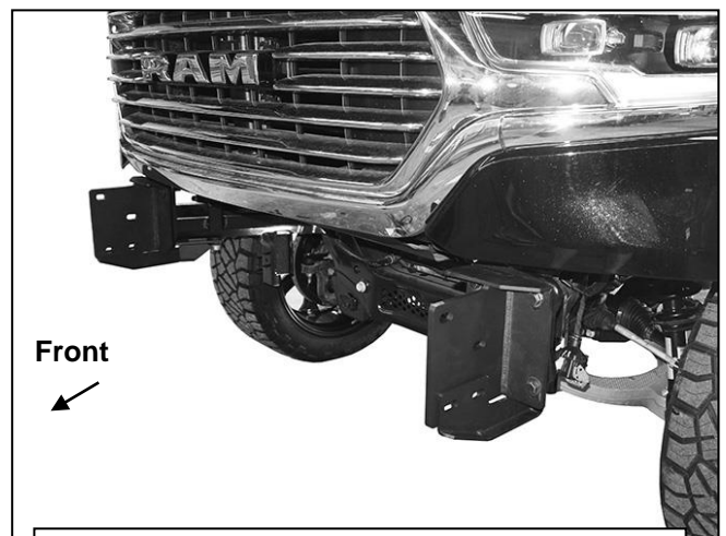
(Fig 8) Frame and Support Brackets installed
