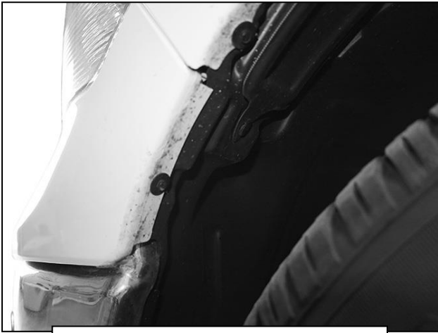
(Fig 1) Remove hardware attaching plastic fender liner to fender
