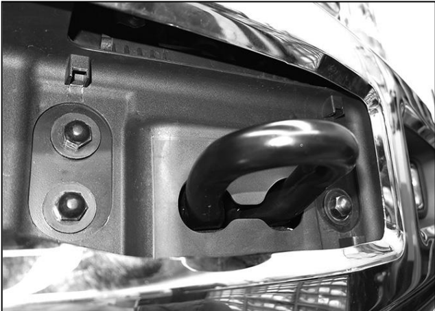
(Fig 6) Remove bumper bolts (driver side pictured)
