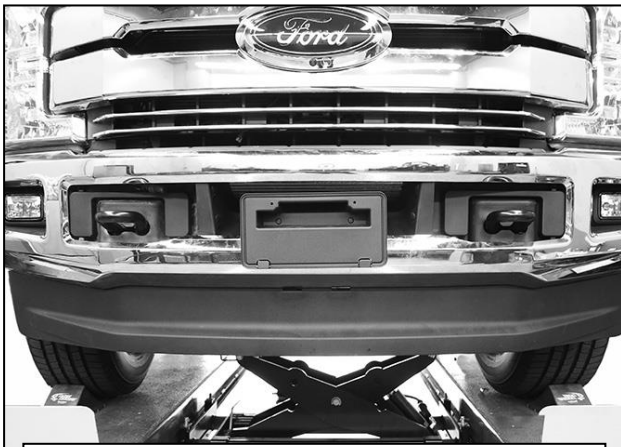
(Fig 3) Remove plastic air dam from bumper
