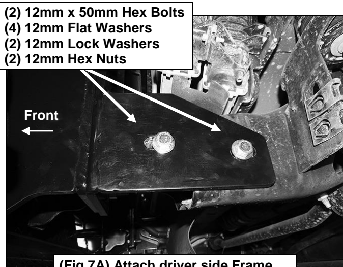
(Fig 7A) Attach driver side Frame Bracket to outside of frame channel
