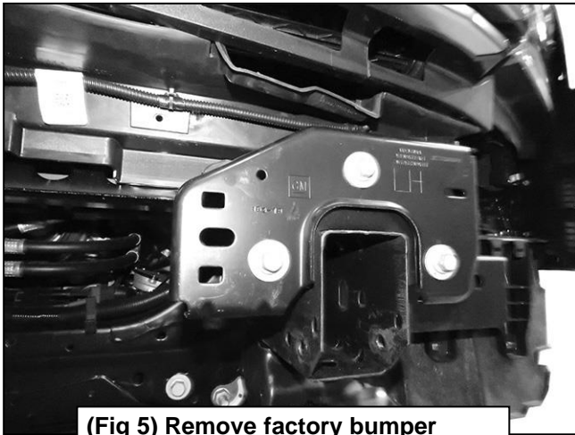
(Fig 5) Remove factory bumper brackets and tow hooks if equipped
