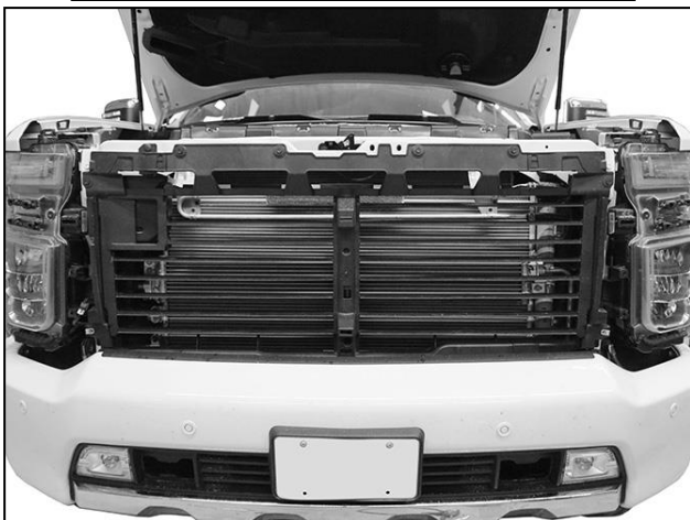
(Fig 7) Grille and fascia removed
