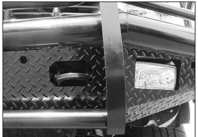
(Fig 11B) Reinstall tow hooks with factory hardware
