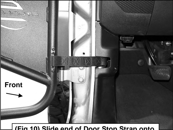
(Fig 10) Slide end of Door Stop Strap onto bracket )driver/left front Door pictured)
