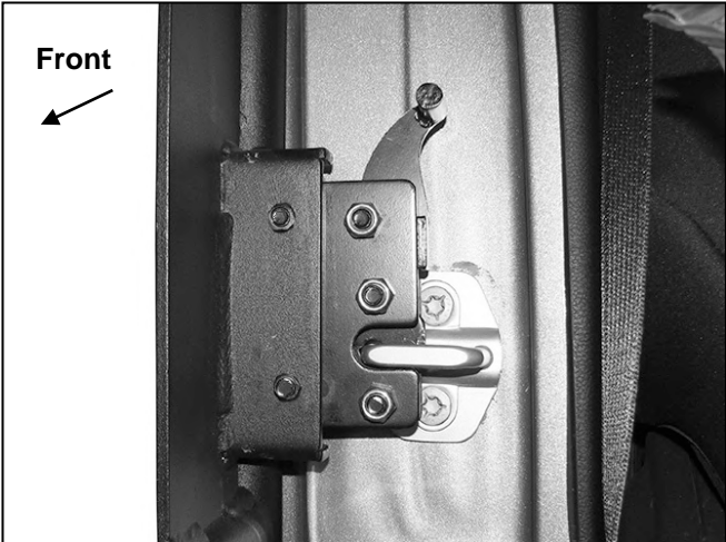
(Fig 12) Adjust Door and Latch assembly for proper operation before fully tightening hardware. Make sure door latch fully closes against striker
