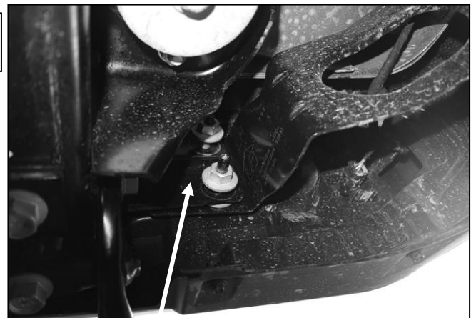
(Fig 4) Loosen the factory bumper bolts, (2 per side) to help reinstall L-shaped Bracket
