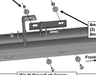
(Fig 9) Driver/Left Center Support Bracket installation
