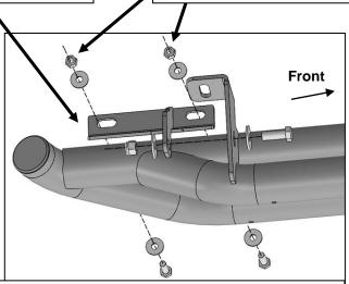
(Fig 10) Driver/Left Rear Support Bracket installation (Driver/Left Rear Support Bracket is the same as the Passenger/Right Front and Center Support Brackets)
