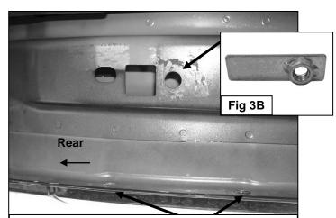
(Fig 3A) Line up Nut Plate with the hole in between the pair of (2) holes on the pinch weld
