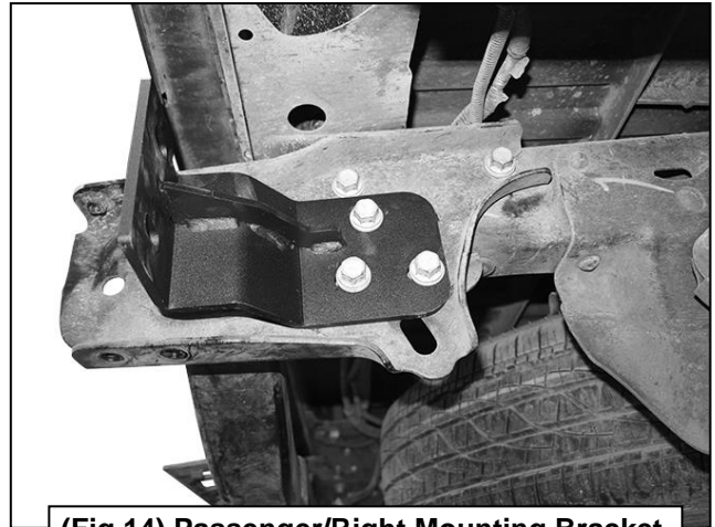
(Fig 14) Passenger/Right Mounting Bracket attached (Model with hitch pictured)
