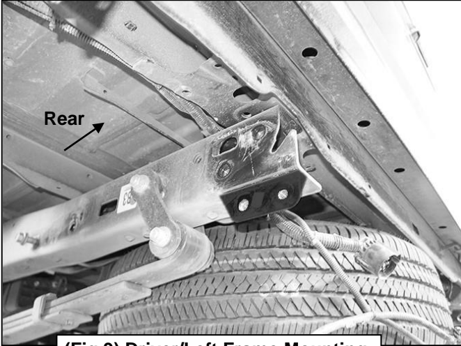
(Fig 9) Driver/Left Frame Mounting Location with the Support Bracket attached (Models without hitch)
