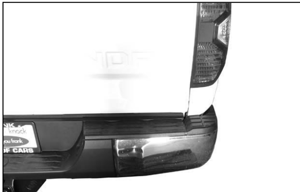
(Fig 3) Use a flat blade screwdriver to pry the plastic cover from the top of edges of the bumper
