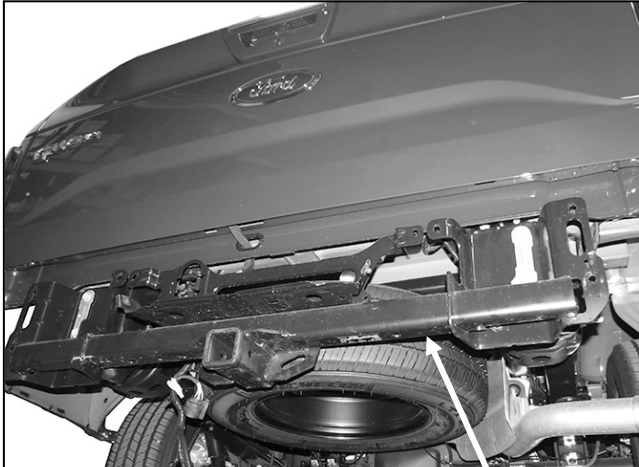
(Fig 12) Reinstall integrated receiver hitch/bracket assembly on models with "HD Towing" package
