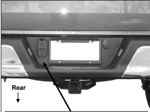
(Fig 1) Unplug and remove 7-wire trailer plug
