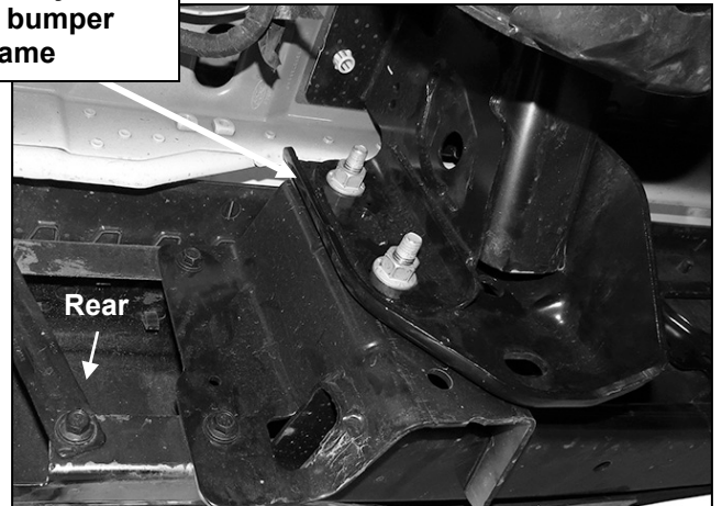
(Fig 3B) Remove the factory hex nuts attaching bumper assembly to frame. STD tow package model pictured (no receiver hitch)
