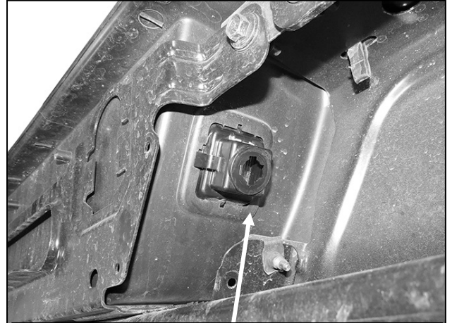
(Fig 2) Unplug and remove license plate lights
