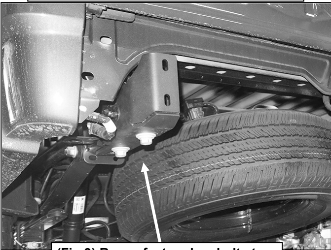
(Fig 9) Reuse factory hex bolts to attach Brackets to bottom of frame
