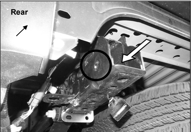
(Fig 5) Insert 10mm Single Bolt Plate into open end of frame and out hole in side of frame
