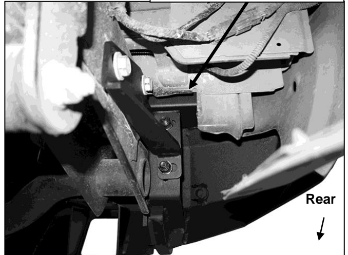
(Fig 10) Attach Bumper to Frame Brackets (driver/left side pictured from below)
