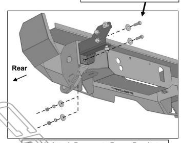
(Fig 11) Attach Bumper to Frame Brackets
