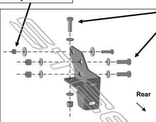
(Fig 6) Attach passenger/right Frame Bracket mounting holes in frame and hitch if equipped
