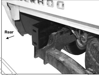
(Fig 7) Driver/left Bracket installed on Model with receiver hitch
