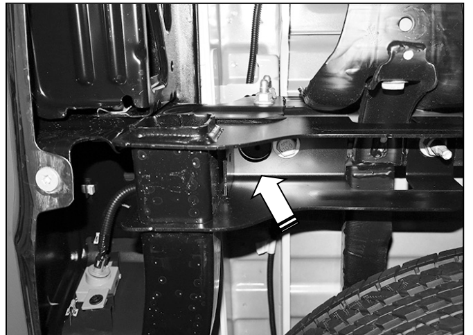
(Fig 4) OPTION: Access rear bed mounting bolts through hole in frame. Remove bed bolts and raise bed to remove bumper with brackets attached
