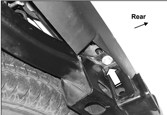
(Fig 1) Factory bumper may be attached to top of tow hitch. Remove factory hex bolts as required.
