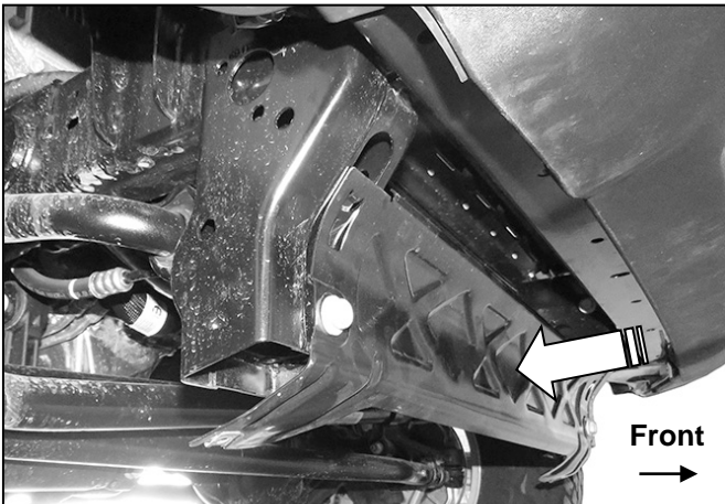
(Fig 1) Remove splash guard and bracket (arrow)
