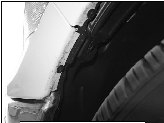
(Fig 1) Remove hardware attaching plastic fender liner to fender
