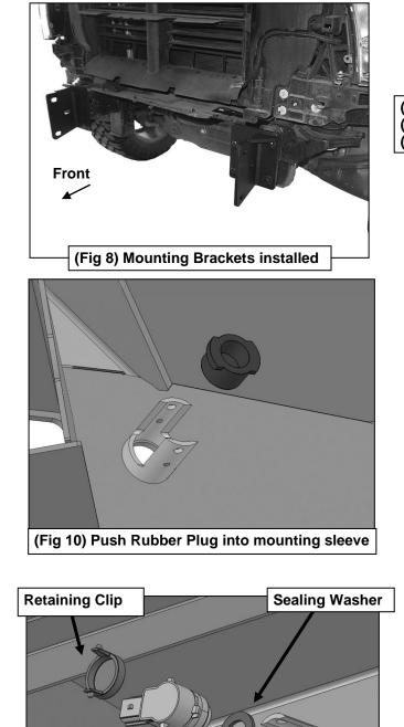
(Fig 12) Push sensor with Sealing Washer into sleeve
