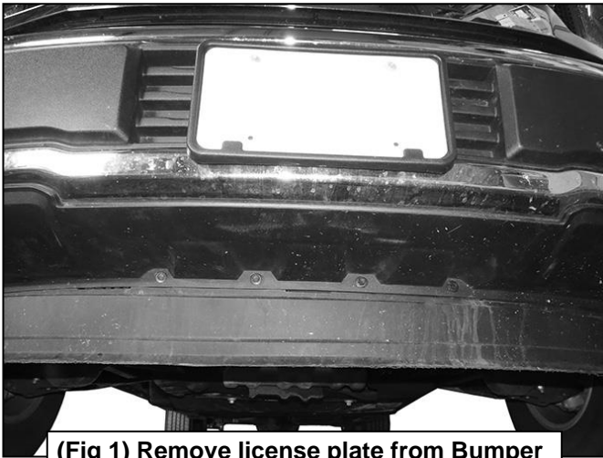
(Fig 1) Remove license plate from Bumper
