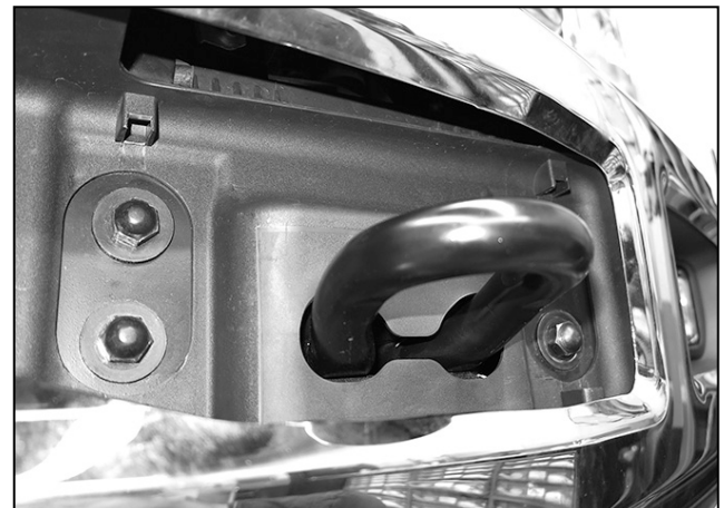
(Fig 4) Remove bumper bolts (driver side pictured)
