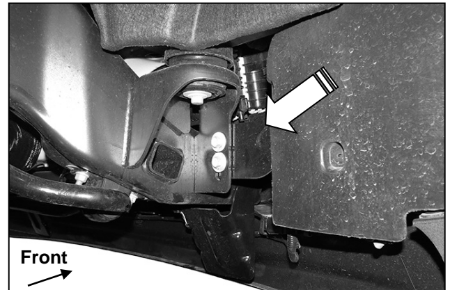
(Fig 2) Remove outer bumper support brackets between frame and bumper (arrow)
