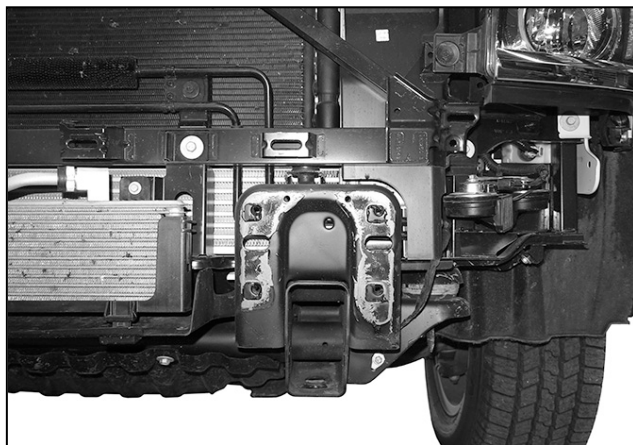
(Fig 5) Remove bumper brackets and tow hooks
