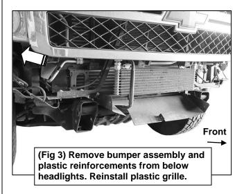
Remove bumper bolts from top of bumper brackets (arrows) to remove bumper
