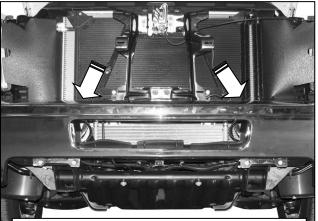
(Fig 2) Remove grille to access bumper bolts. Bumper pictured without lower air dam for instruction purposes-do not remove lower air dam for installation.
