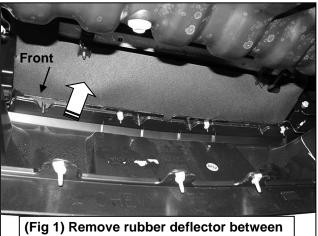
back of bumper and bottom of radiator. Pictured from below-under front bumper.
